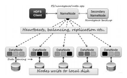
Fig. 1. HDFS frame structure
