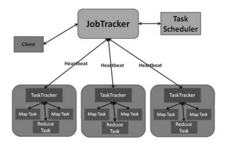
Fig. 2. Diagram of the Map/Reduce framework
